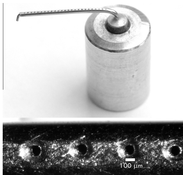
Fig. 2. Photograph of the RFQ nozzle. (Inset) micrograph of the holes in the nozzle tube with a scale bar.
